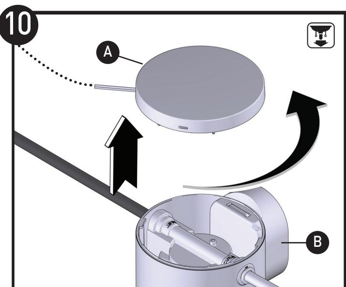
Remove Manifold Cap (A) from Manifold (B) by gently unscrewing the cap.
