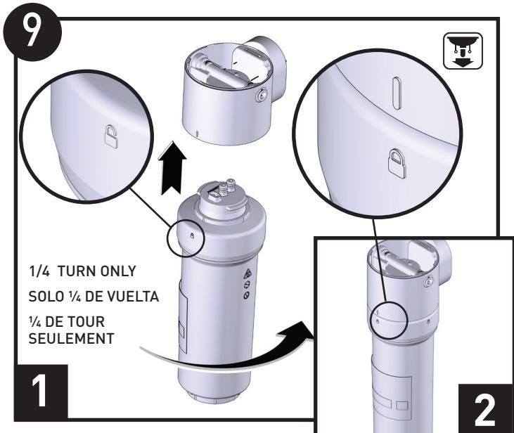
1. Install Sump Assembly into Mounting Manifold by inserting the product up and turning 1/4 to secure.
