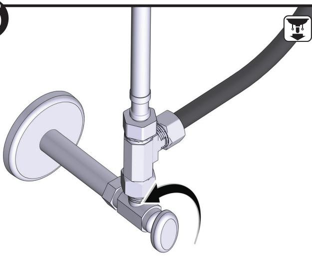
Turn on cold water supply. Let water run for 10 minutes for flushing of any debris.
