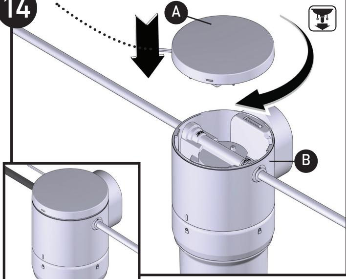
Install Manifold Cap **(A)** into Manifold **(B)** by placing Cap on top of Manifold and gently turning until secure.
