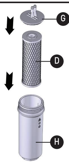
Remove Housing waterway (G) and Filter (D) from Filter housing (H). Discard and throw away old filter unit.
