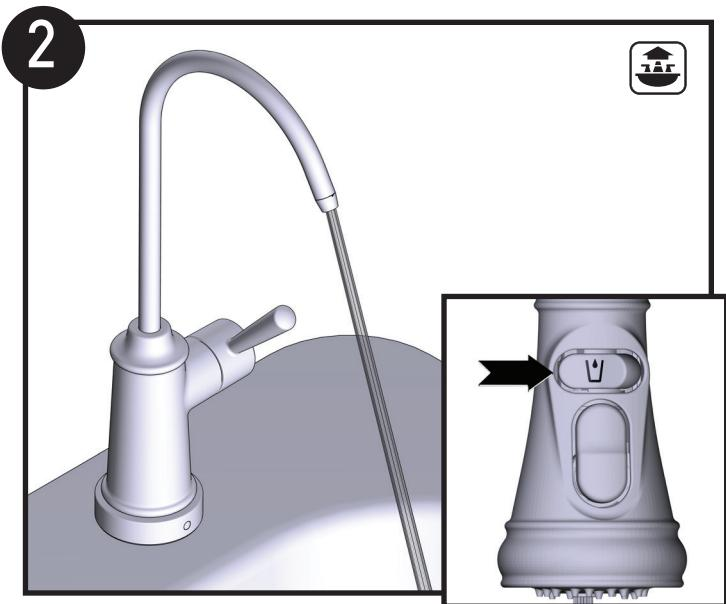
Activate filtered water flow (method will vary based on faucet style). Allow sufficient time for faucet to drain any remaining water.
