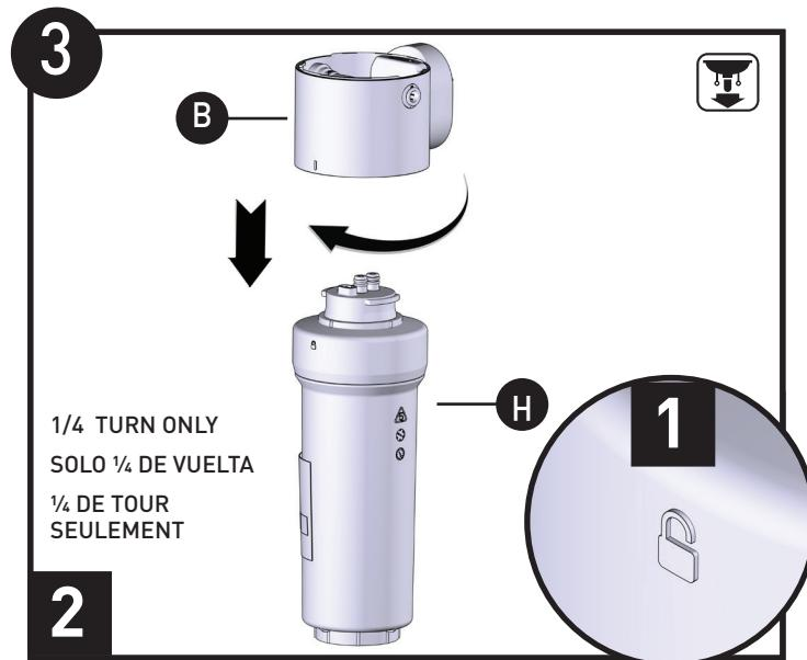
1. Rotate the installed Filter Housing Unit (H) to ensure the unlocked mark aligns with the manifold (B).
