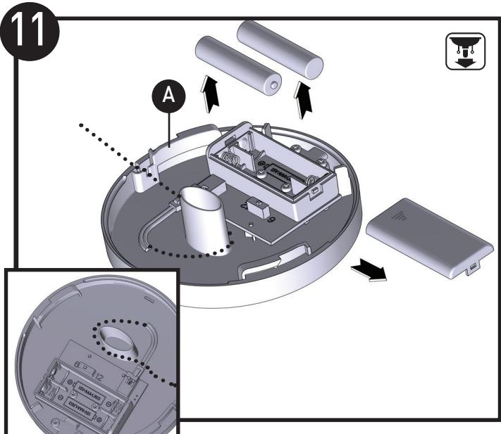
Remove battery box cover and remove existing 2 AAA batteries from the Manifold Cap (A).
