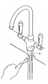
5. Check the position on the sink of the faucet, then tighten the nut with a 13mm wrench.
