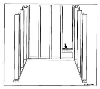
Construct the bench seat framework, as shown, using 2 x 4 wood or steel studs. The framework for the seat must be 11-3/4" deep and can be up to 47-1/2" long, depending on your application.
