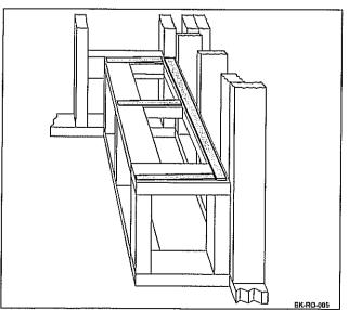
Install 1/2" moisture-resistant cement board or greenboard over all the surfaces of the seat area (1, 2, & 3). Follow the wall board manufacturer's recommendations for installation.
