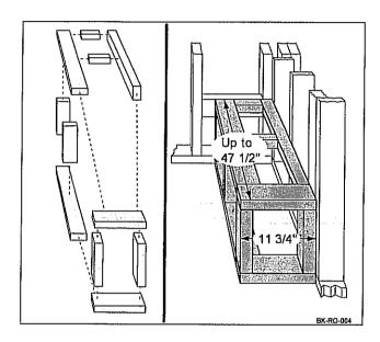
3. In order to eliminate standing water on the bench seat, cut and place three, 2" wide shims on top of each 2 x 4, as shown. Standard shim stock works well for these shims. The shims should be 1/8" thick and taper down to nothing. Also, place a 1/8" thick shim along the wall to completely support the back of the seat.
