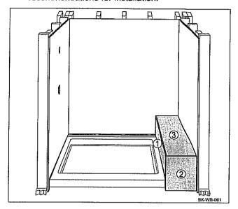
Apply a coat of water or oil-based primer/sealer to all the surfaces of the cementboard or greenboard (follow the manufacturer's instructions). Allow the primer to dry thoroughly before applying any clear silicone.
